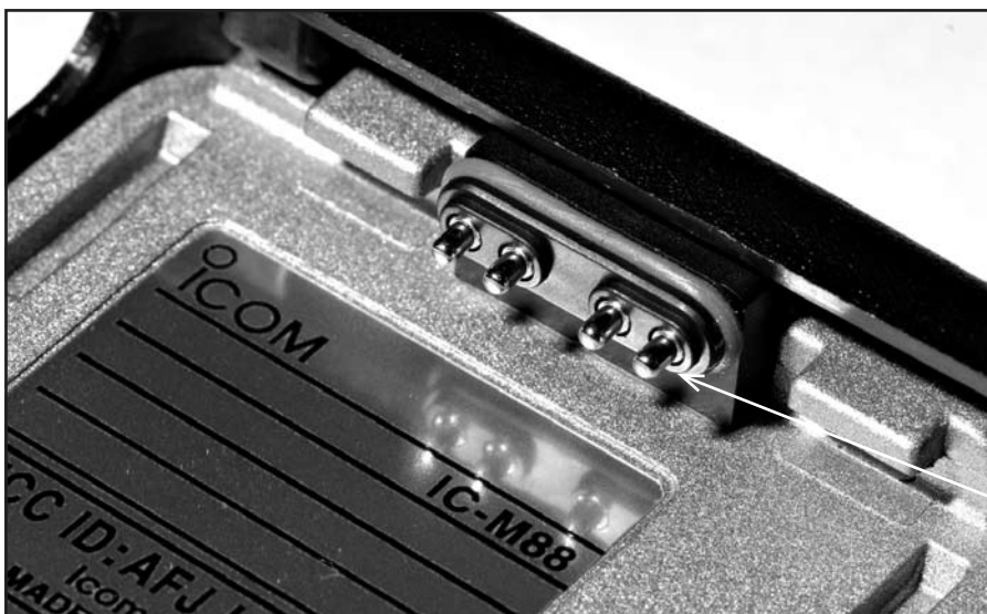
Left: A few drops of water got inside of the Icom IC-M88's battery compartment after our dunk test, but a gasket protects the battery-to-radio connection.
