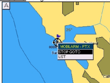
Figure 16.4.1b - Example of Stop Goto PTX on CP180/CP180i
