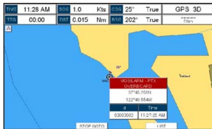
Figure 16.4.1c - Example of Stop Goto PTX on CP300/CP300i
