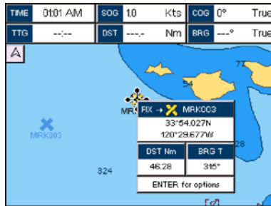
Figure 7.1.1a - Moving Mark or Waypoint (2)
