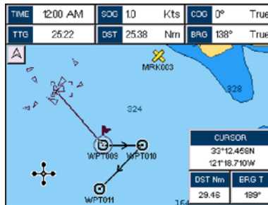
Figure 9.6.0a - GOTO ROUTE procedure (2)
