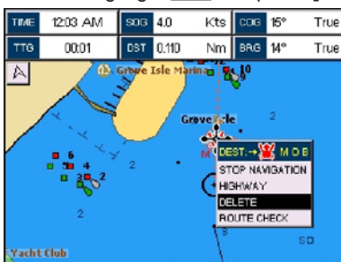
Figure 8.1 - Deleting MOB point
