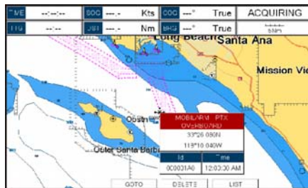
Figure 16.4 - Example of PTX information window on CP300/CP300i
