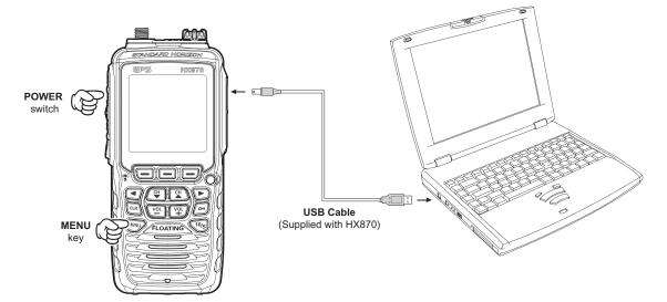
The transceiver will beep and display "CP MODE" on the LCD.
