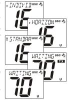
If the reply signal is not received, the transceiver will transmit again.
