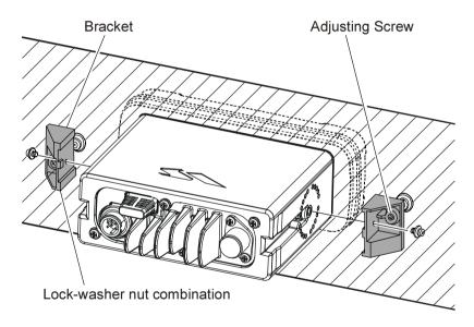
Figure 4. MMB-84 Flush Mount Installation
