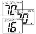
7. When an individual call acknowledgment is received, the established channel is automatically selected and a ringing tone sounds.
