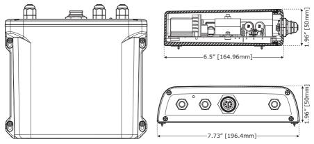
Figure 4 - FF525 Dimensions [inch/mm]
