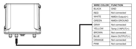
Figure 2.4 - The FF525 Optional Connections
