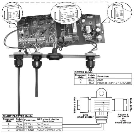
Figure 2.3.1b - Internal connections
