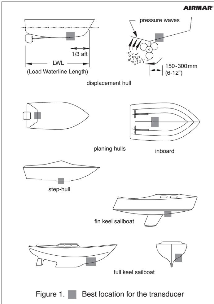
Figure 1. ■ Best location for the transducer
