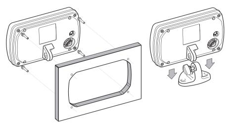
Figure 4.1.1 - Installing/removing chartplotter
