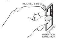
Figure 4.1.7.1 - Inserting/Removing C-CARD (I)
