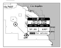
Figure 4.5.1 - Placing Destination on Cursor
