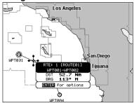
Figure 4.4.1.6 - Placing Waypoint between two existing ones (I)
