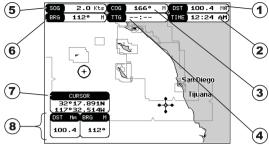
Distance and Bearings from Fix to Cursor (if the Fix is NOT received, DST and BRG are empty)
