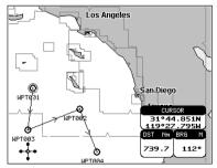
Figure 4.4.1.6b - Placing Waypoint between two existing ones (III)
