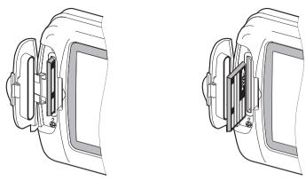
Figure 4.1.7.1a - Inserting/Removing C-CARD (II)
