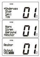
5. To exit the "FOG HORN" mode and return to radio operation mode, press the [F] key followed by the [9(FOG)] key again.
