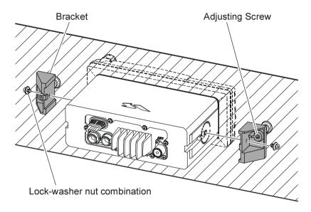
Figure 2. MMB-84 Flush Mount Installation
