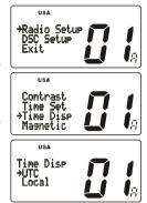
In the local time mode, the display shows the time by the 12-hour system. Meanwhile, the display shows the time by the 24-hour system in the UTC mode.
