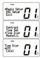
n the local time mode, the display shows the time by the 12-hour system. Meanwhile, the display shows the time by the 24-hour system in the UTC mode.
