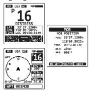
To transmit a DSC distress message, lift the red spring-loaded DISTRESS cover on the right side of the transceiver, then press and hold the DISTRESS key (see section "10.2.1 Transmitting a DSC Distress Alert" for details). The nature of the Distress Alert is automatically set to "MOB".
