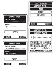
If a mistake was made entering in the name, press the  $[CH \ ]/[CH \ ]/[\ ]/[\ ]/[\ ]/[\ ]$  key to select " $\leftarrow$ " or " $\rightarrow$ ", press the [SELECT] soft key until the wrong character is selected, then perform steps 3 and 4.
