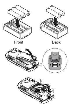
To remove the battery case, turn the transceiver **OFF**, open the battery cover, then push and lift up the bottom end of the battery case.
