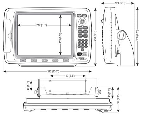
Figure 2.0.0 - Chart plotter Dimensions [mm/inch]
