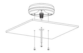
Figure 2.1b - Installing the Smart DGPS WAAS antenna (III)
