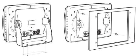
Figure 2.0 - Installing/removing chart plotter
