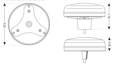
Figure 2.1.1 - Smart DGPS WAAS antenna Dimensions
