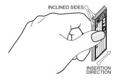
Figure 2.7 - Inserting C-CARD (I)
