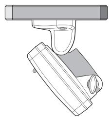
Figure 2.0a - Optional overhead mounting bracket
