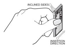
Figure 2.4 - Inserting C-CARD (I)
