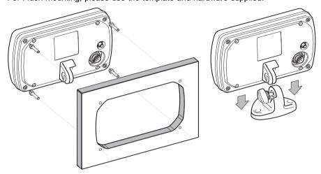
Figure 2.0 - Installing/removing chart plotter
