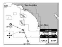
Figure 3.8.3a - Placing Waypoint between two existing ones (II)
