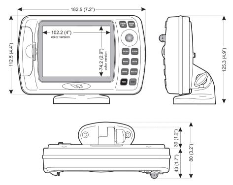
Figure 3.13 - Chart plotter Dimensions [mm/inch]
