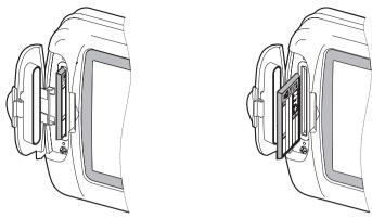
Figure 2.4a - Inserting C-CARD (II)
