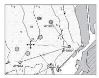
Figure 4.4.1.6a - Placing Waypoint between two existing ones (II)
