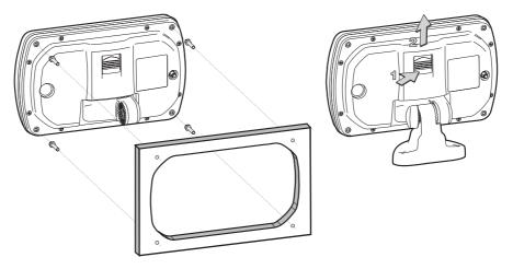
Figure 4.1.1 - Installing/removing chartplotter
