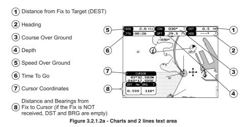
As in the previous Figure 3.2.1.2, when in <u>Home</u> mode the coordinates field (a) shows ship's coordinates; the six fields (a), (a), (a), (b), (c) are selectable fields as described in the previous Section 3.2.1.
