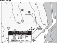
Figure 4.4.1.6 - Placing Waypoint between two existing ones (I)
