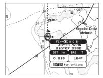
Figure 4.6.1 - Placing MOB
