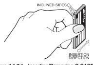
Figure 4.1.7.1 - Inserting/Removing C-CARD (I)
