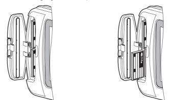
Figure 4.1.7.1a - Inserting/Removing C-CARD (II)
