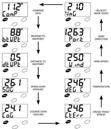
Note: If a depth, speed, or wind instrument other than the 150 series is connected, the data will be shown by using the NMEA key.
