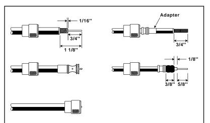
To get your coax cable through a fitting and into your boat's interior, you may have to cut off the end plug and reattach it later. You can do this if you follow the directions that come with the connector. Be sure to make good soldered connections.
