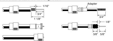
To get your coax cable through a fitting and into your boat's interior, you may have to cut off the end plug and reattach it later. You can do this if you follow the directions that come with the connector. Be sure to make good soldered connections.
