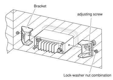
Figure 3. CMB16 Flush Mount Installation
