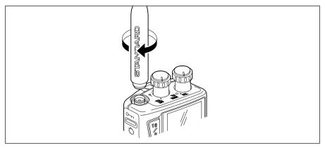
Figure 4. Antenna Installation
