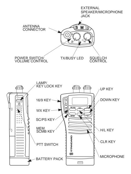
Figure 1. Controls and Connectors
