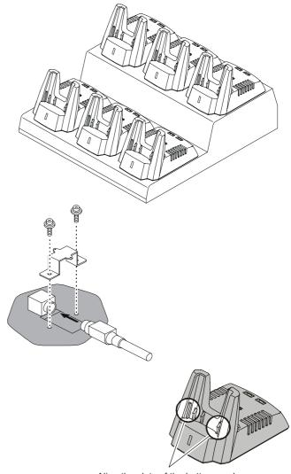
Align the slots of the battery pack with the guides in the nest of the **VAC-6010** 6-Unit Multi Charger.
