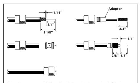
To get your coax cable through a fitting and into your boat's interior, you may have to cut off the end plug and reattach it later. You can do this if you follow the directions that come with the connector. Be sure to make good soldered connections.
