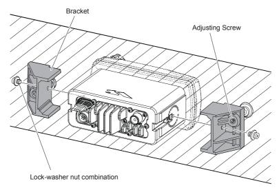
Figure 2. MMB-84 Flush Mount Installation
