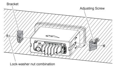
Figure 2. MMB-84 Flush Mount Installation
