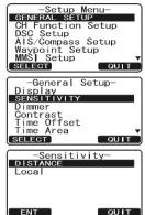
To return to normal sensitivity, repeat the above procedure, rotating the **CHAN-NEL** knob to select "DISTANCE" in step "5" above.
