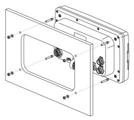
Figure 2.2 - Example of Flush installation
