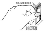
Figure 5.1 - Inserting C-CARD
