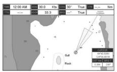
Figure 13.3 - Grounding Alarm
