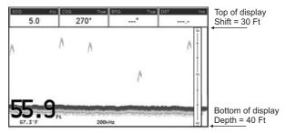
Figure 17.9.2 - Example of Depth and Shift
