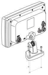
Figure 2.1 - Example of Bracket installation
