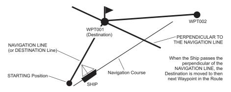
Figure 9 - Example to show how the plotter switches from one Waypoint to another
