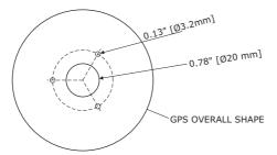
Figure 2.3.0a - Installing the External GPS antenna (II)
