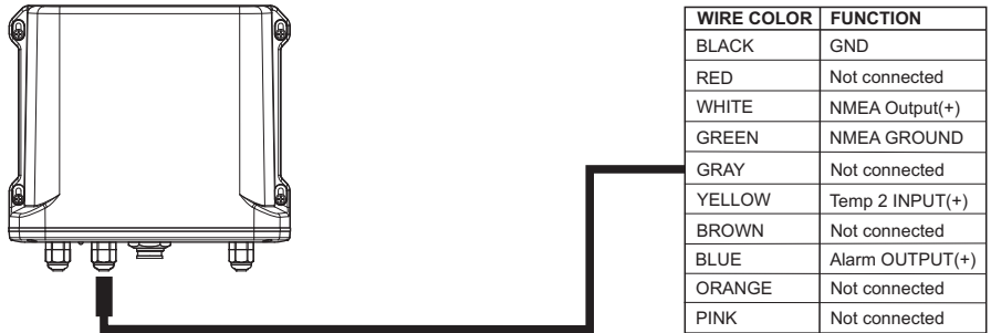
Figure 2.4 - The FF525 Optional Connections
