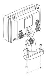
Figure 2.1 - Example of Bracket installation on CPF190i
