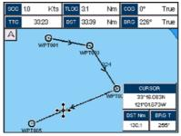
Figure 9.5 - Inserting Waypoint procedure (1)
