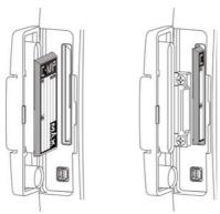
Figure 5.1a - Inserting C-CARD (details)
