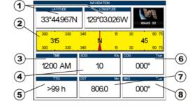
Figure 12.2a - Navigation page with Compass Tape
