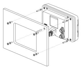
Figure 2.2 - Example of Flush installation on CPF190i
