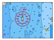
Figure 13.3 - Grounding Alarm
