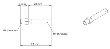
Figure 2.2.0 - Mounting Screws
