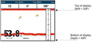
Figure 17.8.2 - Example of Depth and Shift
