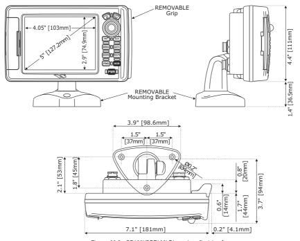
Figure 20.2 - CP190i/CPF190i Dimensions [inch/mm]
