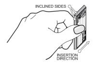
Figure 5.1 - Inserting C-CARD
