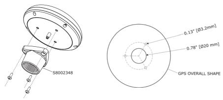
Figure 2.3.0 - Installing the External GPS antenna
