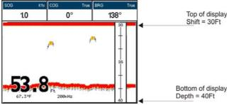
Figure 17.9.2 - Example of Depth and Shift
