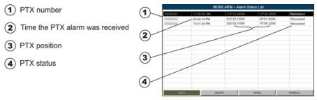
Figure 16.4.2 - Example of MOBilarm PTX List page on CPF300i
