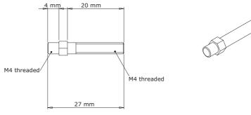
Figure 2.2.0 - Mounting Screws
