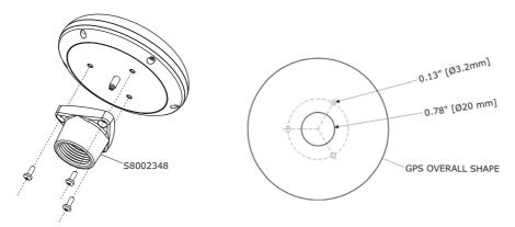
Figure 2.3.0 - Installing the External GPS antenna (I)
