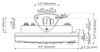
Figure 20.1 - CPF300i Dimensions [inch/mm]
