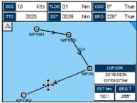
Figure 9.5 - Inserting Waypoint procedure (1)
