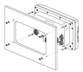
Figure 2.2a - Example of Flush installation on CPF300i
