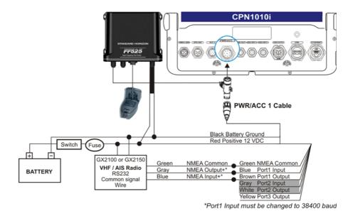
() Gray and White wires should not be connected to other devices when the FF525 is connected.
