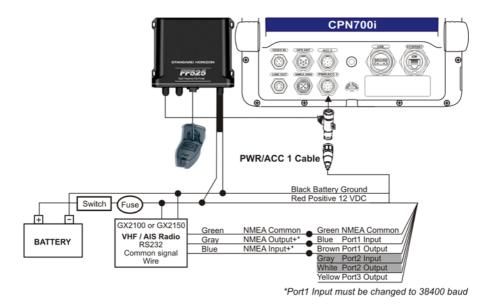
Gray and White wires should not be connected to other devices when the FF525 is connected.
