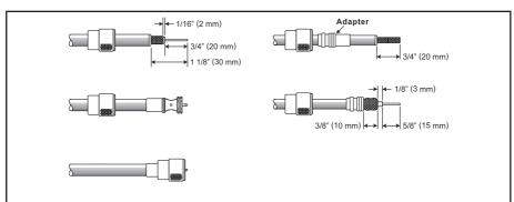
To get your coax cable through a fitting and into your boat's interior, you may have to cut off the end plug and reattach it later. You can do this if you follow the directions that come with the connector. Be sure to make good soldered connections.
