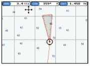
Figure 11.3 - Grounding Alarm
