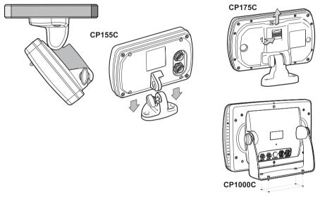
Figure 2.1 - Installing/removing chartplotter (Bracket)
