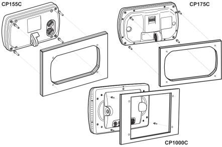
Figure 2.2 - Installing/removing chartplotter (Flush)
