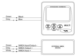
Figure 2.9 - Connecting Digital Instruments/Autopilot/Radar
