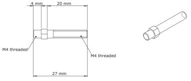
Figure 2.2.0 - Mounting Screws
