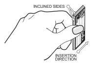
Figure 5.0 - Inserting C-CARD
