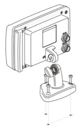
Figure 2.1 - Example of Bracket installation on CP190i
