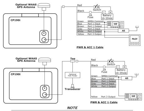
Port2 Input and Output is used by the optional FF525. In the diagram above you will notice Port2 Input and Output wires are shown in gray and not used.
