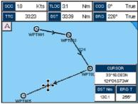
Figure 9.5 - Inserting Waypoint procedure (1)
