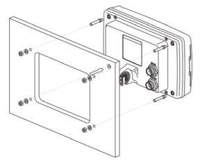
Figure 2.2 - Example of Flush installation on CP190i
