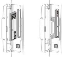
Figure 5.1a - Inserting C-CARD (details)
