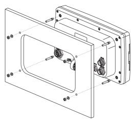
Figure 2.2 - Example of Flush installation
