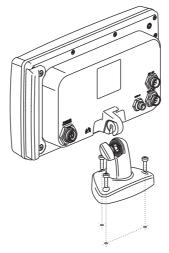
Figure 2.1 - Example of Bracket installation
