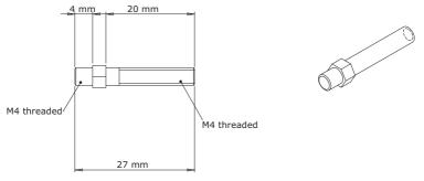
Figure 2.2.0 - Mounting Screws
