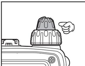
heard, and you may use this noise to set the **VOL** knob for the desired audio level. Press the **MONITOR** button momentarily to silence the noise and resume normal (quiet) monitoring.
