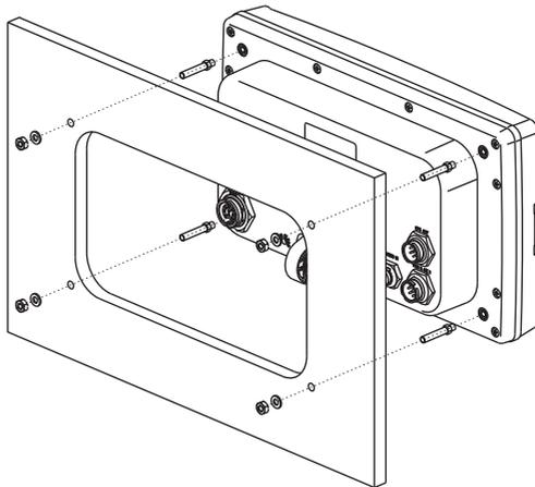
Figure 2.2 - Example of Flush installation
