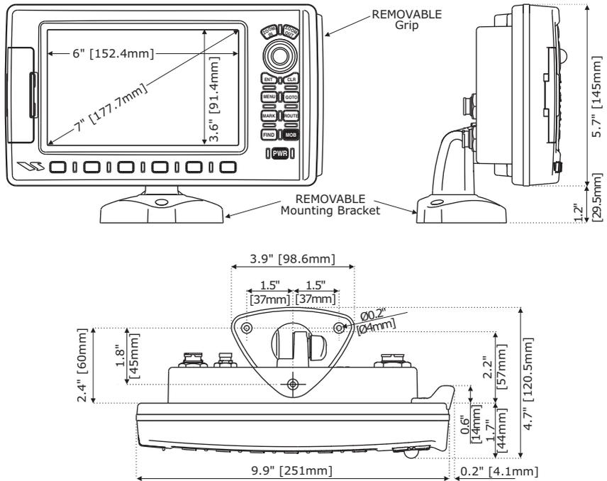
Figure 19.1 - CP390i Dimensions [inch/mm]
