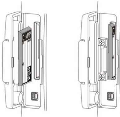
Figure 5.1a - Inserting C-CARD (details)
