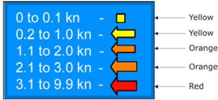
When the GPS Chart Plotter receives a valid position fix, the Tide icons are shown on the charts on the basis of the current date and time: the screen displays and changes arrows as date/time changes.
