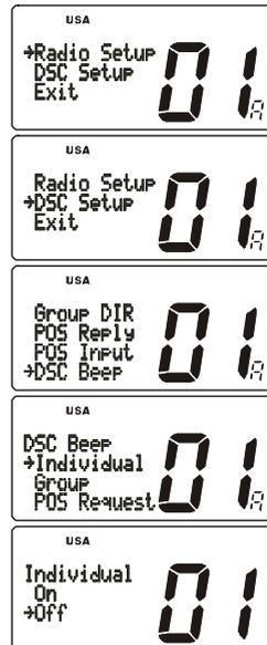
If you wish to return to enabling the ringer tone, just repeat the above procedure, turning the **CHANNEL** selector knob to select “On” in step “6” above.
