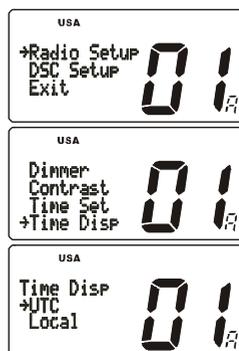
In the local time mode, the display shows the time by the 12-hour system. Meanwhile, the display shows the time by the 24-hour system in the UTC mode.
