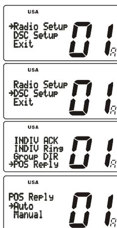
The **GX1500S** has the capability to turn off the Position Request ringer.
