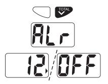
Press and hold both keys for three seconds and the displayed value will begin to flash.
