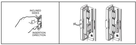
Figure 5.0 - Inserting C-CARD
