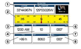
Figure 12.2a - Navigation page with Compass Tape
