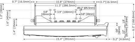
Figure 19 - CP590 Dimensions [inch/mm]
