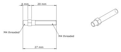
Figure 2.2.0 - Mounting Screws
