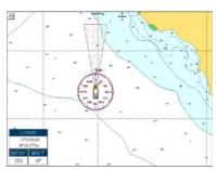
Figure 13.3 - Grounding Alarm
